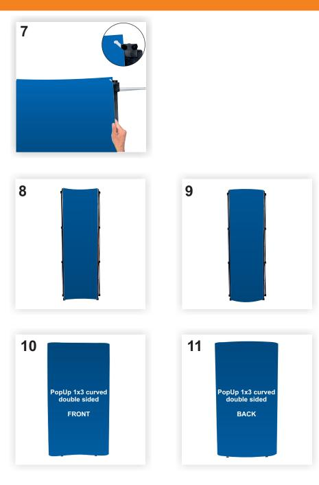
7. Now attach the PopUp graphic (A). The graphic panels are numbered leftto-right to facilitate their positioning on the structure (C). Hang the panels in the cloves at the top of the structure as in the picture. It is recommended to attach the graphic panels starting with the middle panels number 2 and 4.
